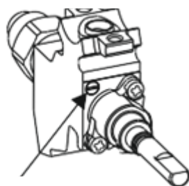
Surub de bypass
