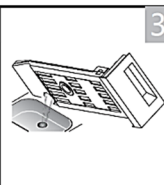
Pull out condensate water
