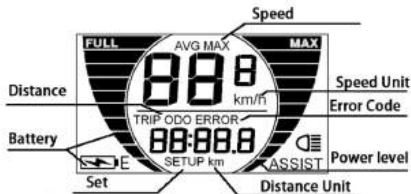
KM529 Monitor Area
