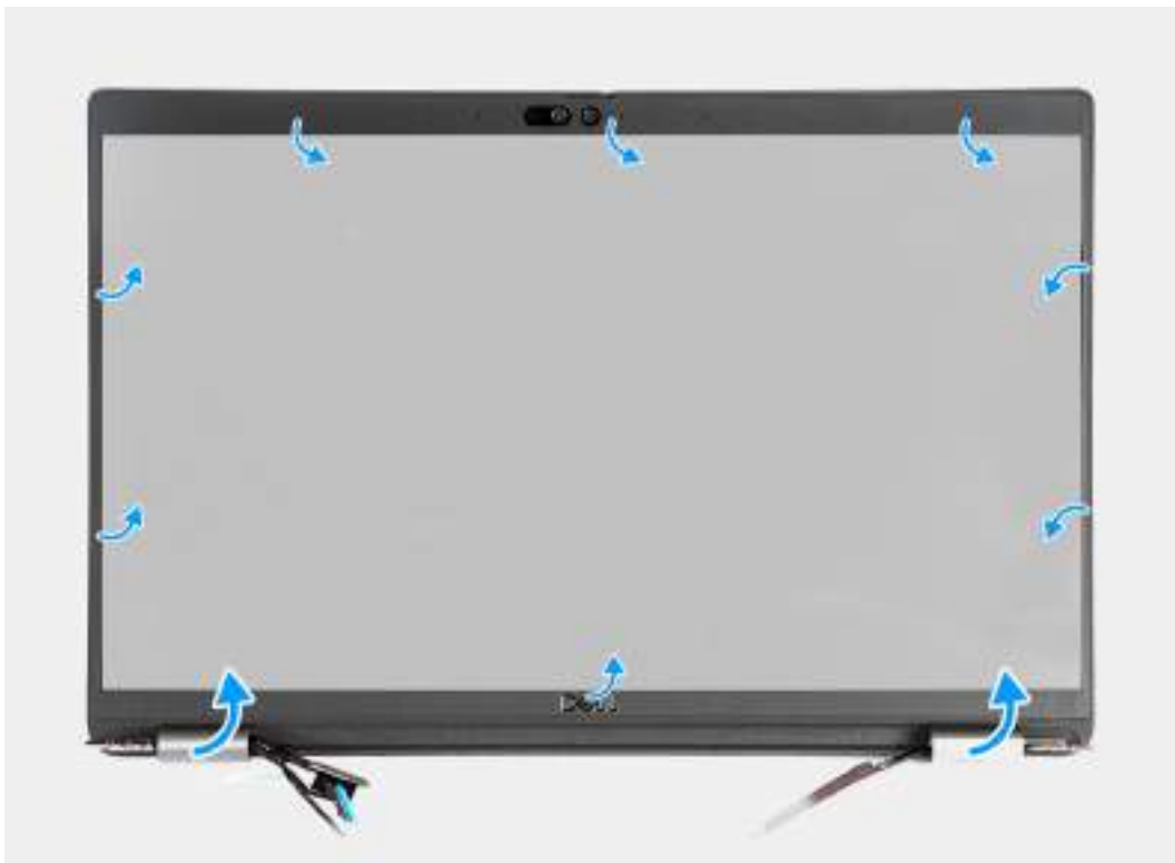
Figure 41. Removing the display bezel
