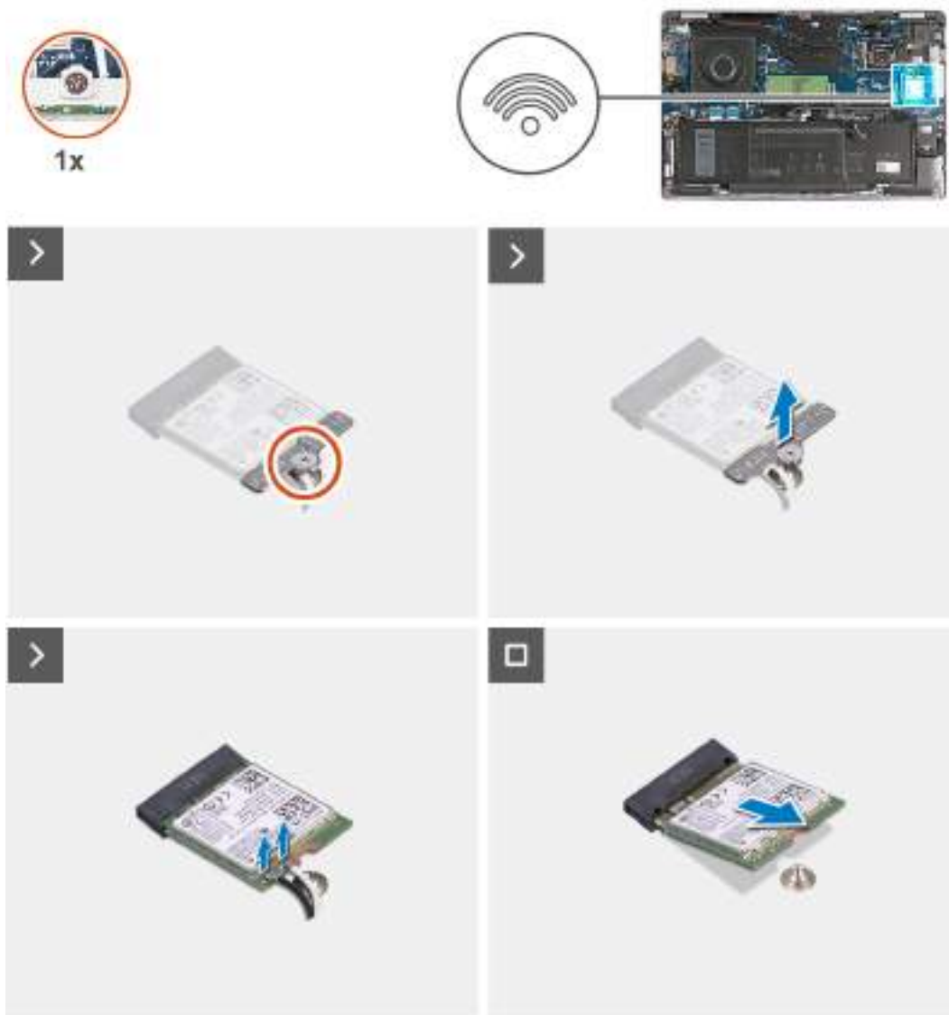
Figure 10. Removing the wireless card
