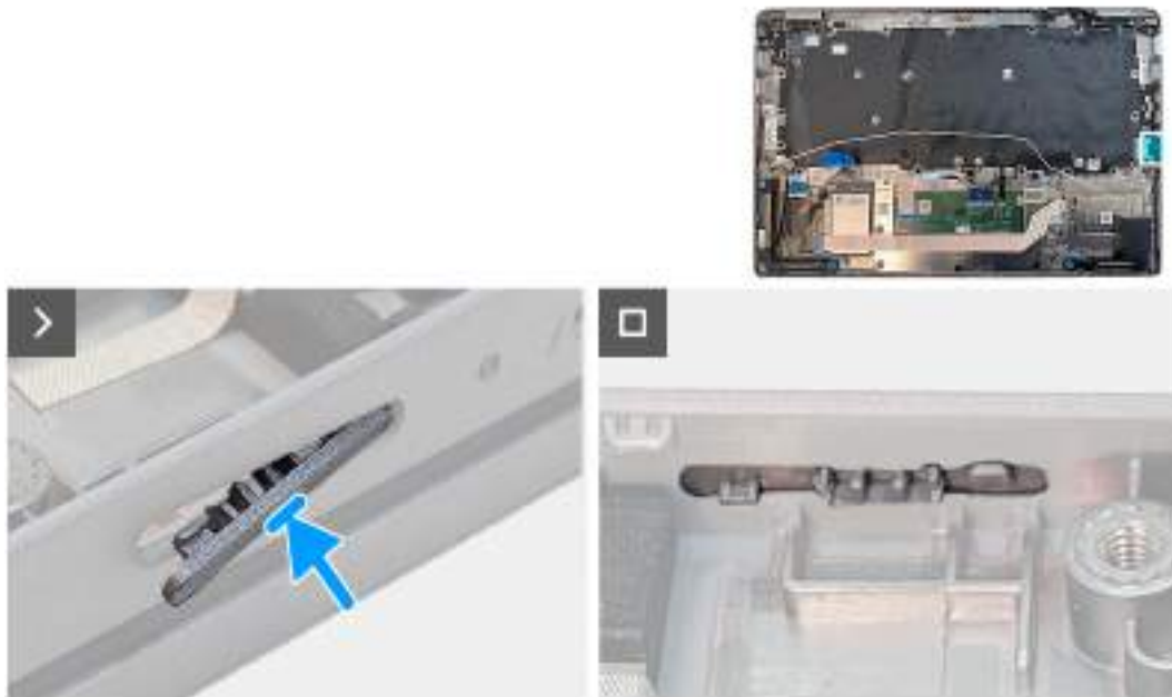
Figure 66. Installing the dummy SIM-card slot filler
