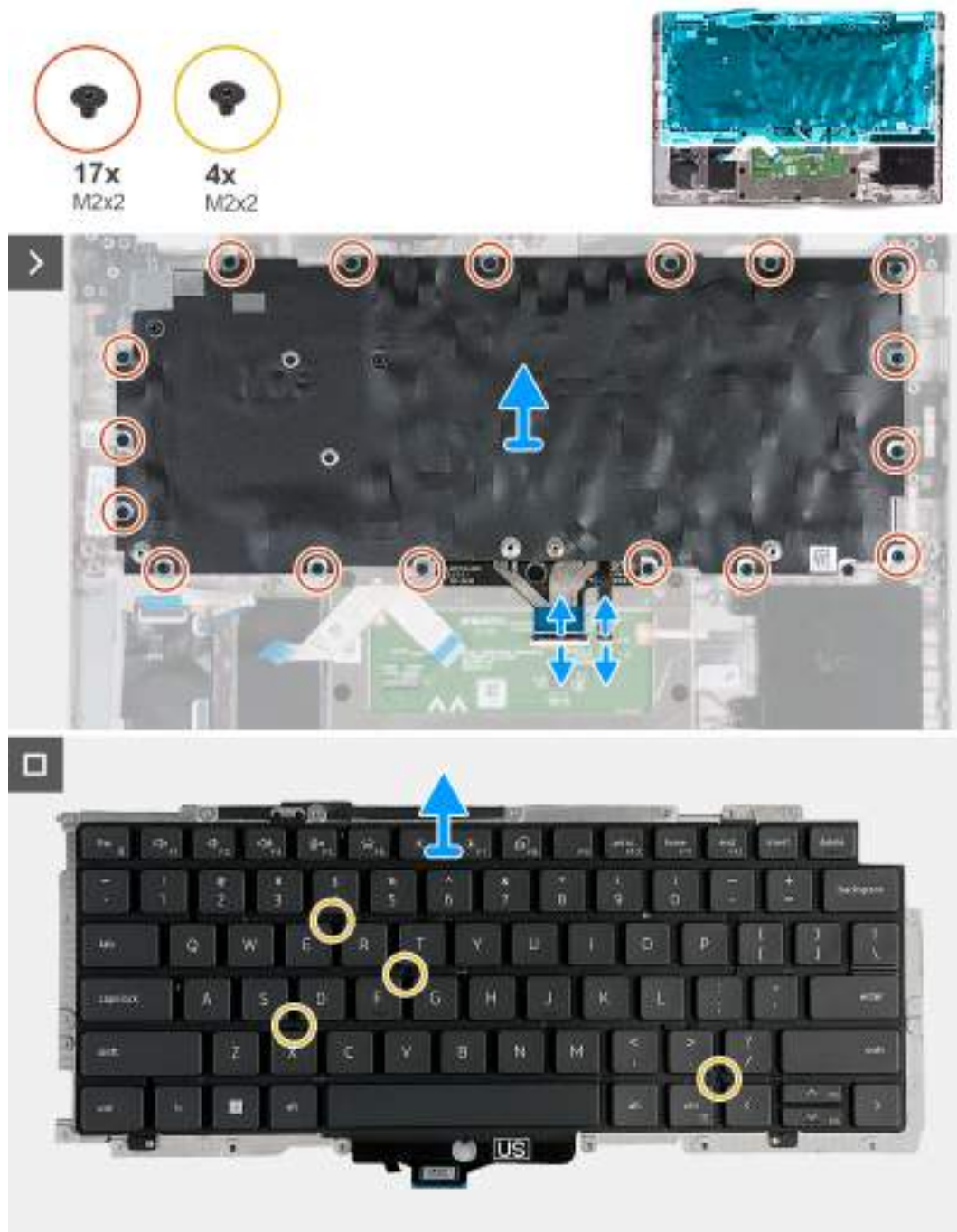
Figure 61. Removing the keyboard
