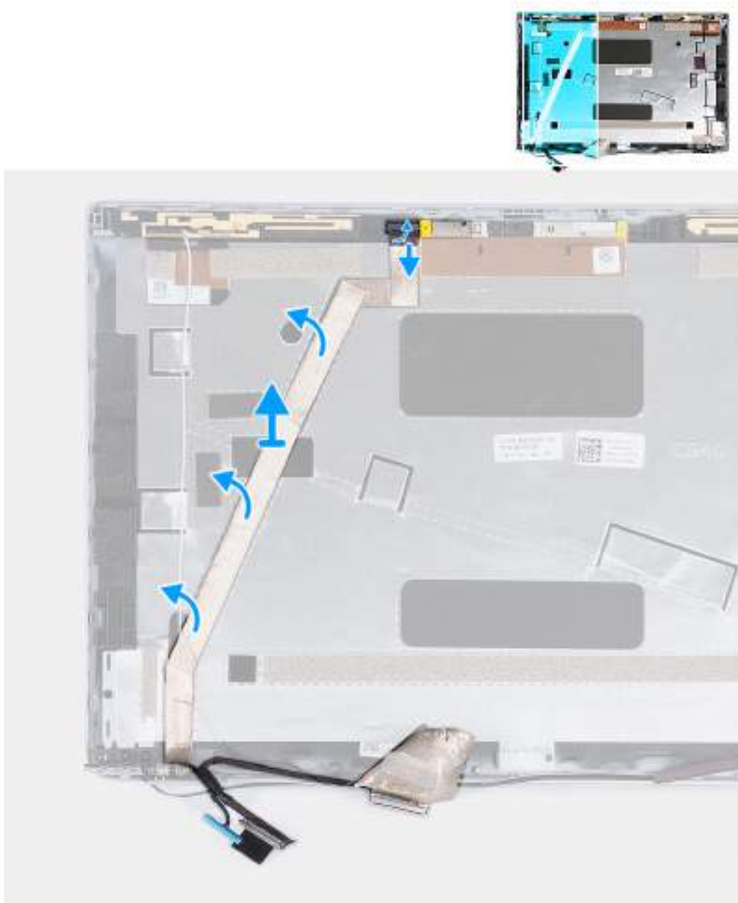
Figure 49. Removing the display cable
