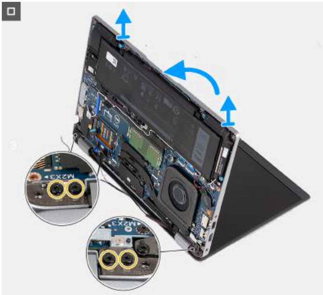
Figure 36. Removing the display assembly - For computers shipped with 5G card
