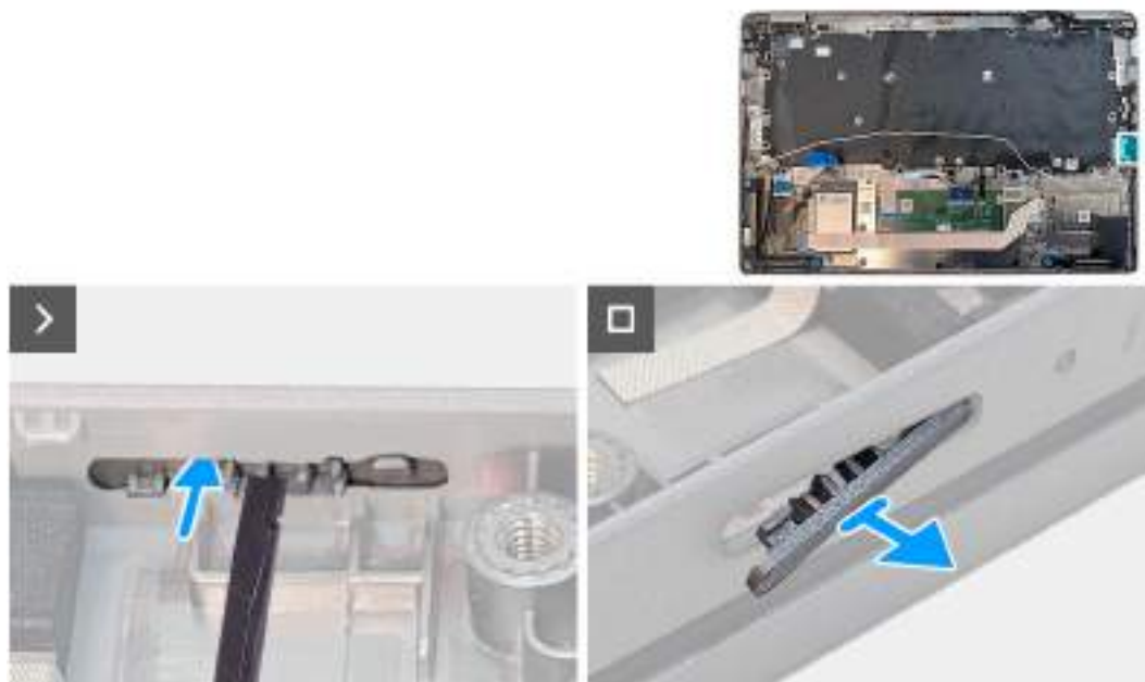
Figure 65. Removing the dummy SIM-card slot filler
