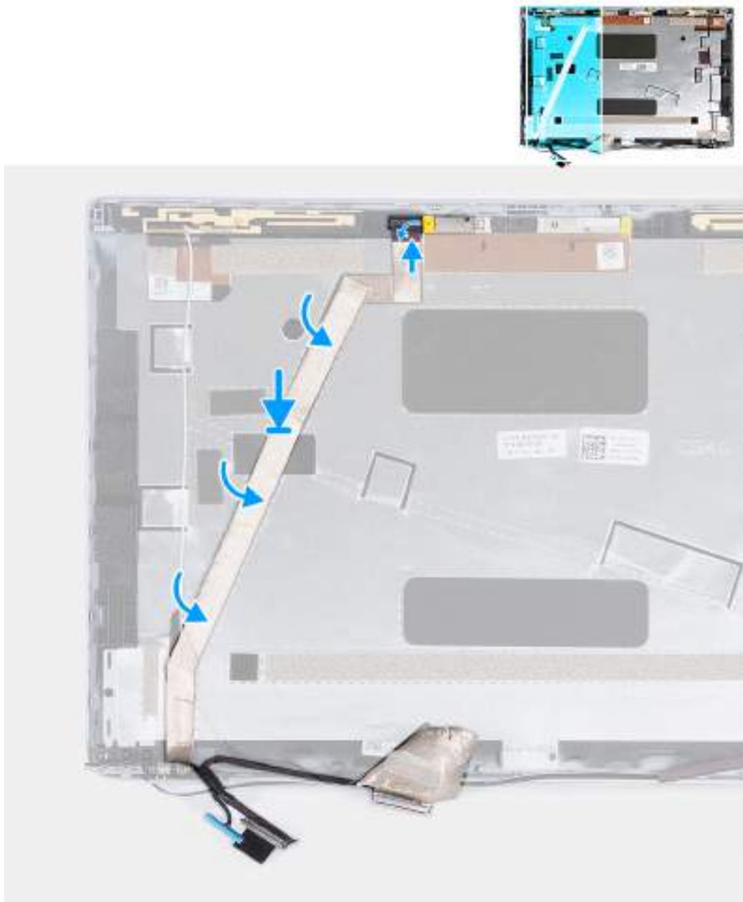
Figure 50. Installing the display cable
