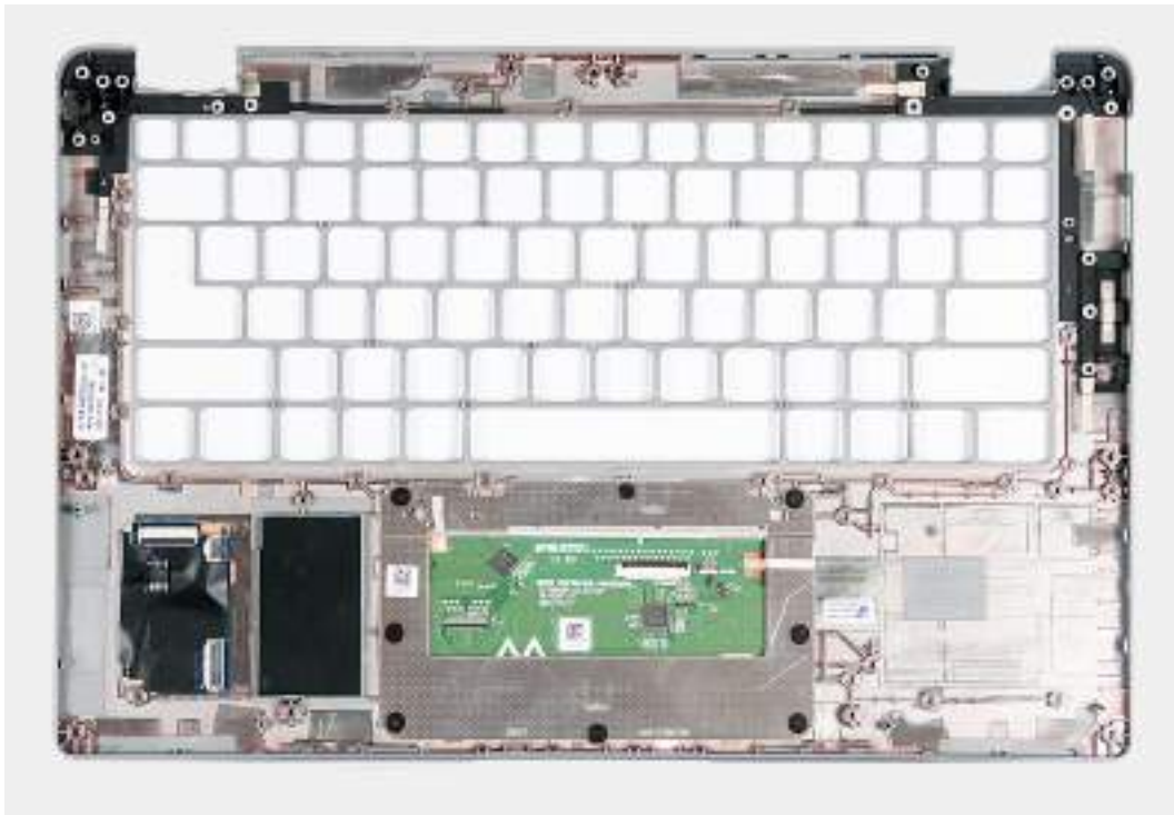
Figure 64. Installing the palm-rest assembly
