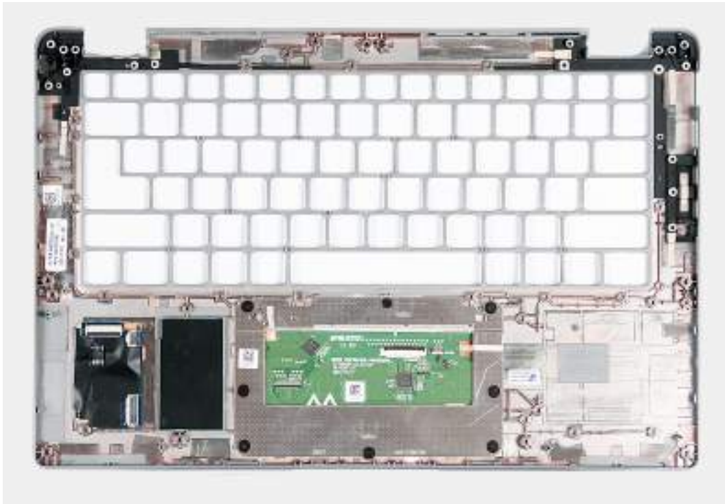
Figure 63. Removing the palm-rest assembly
