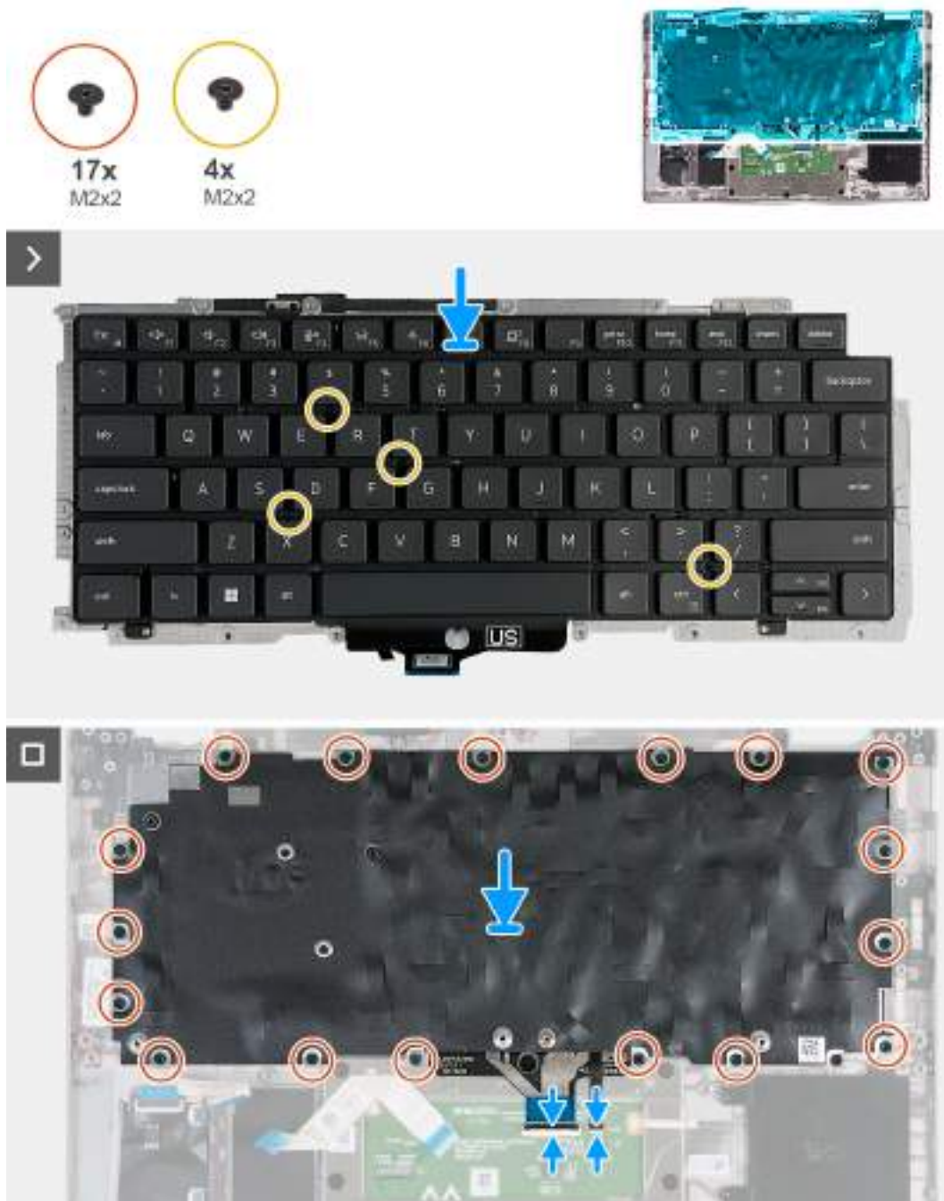
Figure 62. Installing the keyboard
