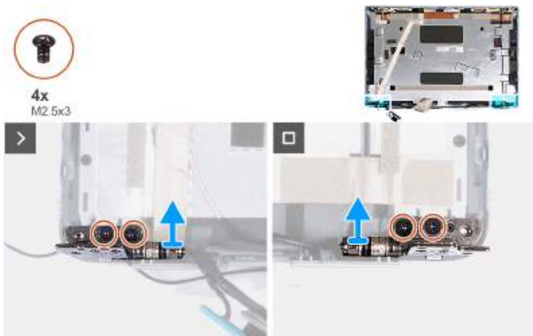
Figure 47. Removing the display hinges
